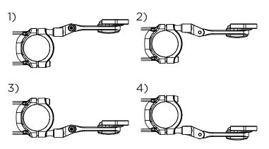
The faceplate mount can be flipped for further customization. If you prefer to flip the faceplate mount, remove the angle adjust screw with a 3mm hex wrench, flip the faceplate mount and reinstall the slotted arm being careful to not damage the angle adjust o-ring. The o-ring can only be installed on the side of the slotted arm with the recess. Tighten the bolt to 3 N-m.
