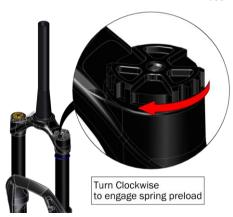
1. Thread push button closed and install cap.
