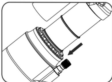
3. Carefully dismount the bike without further compressing the suspension and measure the distance the O-ring has moved.
