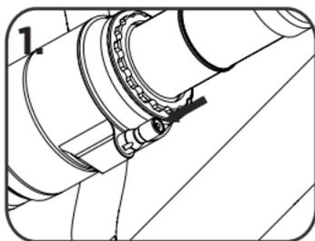
2. Remove the retaining O-ring from the outer air canister
