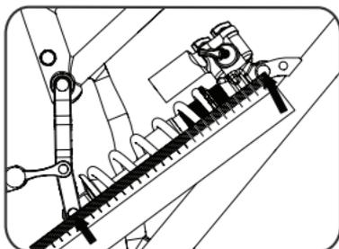
1. With the shock uncompressed, measure the length of your shock from eye to eye.
