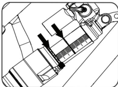
4. This distance is your sag amount and can be converted to a percentage with the following formula.  $(\text{Sag} / \text{Shock Stroke}) \times 100 = \text{Sag Percentage}$  (E.g.  $(16.5\text{mm} / 55\text{mm stroke}) \times 100 = 30\%$ )
