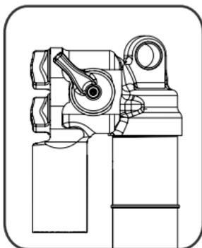
DB Kitsuma features tool free adjustments with all adjusters clearly labeled on the shock. Turning an adjuster counter clockwise will open the circuit which allows more oil flow. (open compression = soft compression / open rebound = fast return speed) Turning an adjuster clockwise will close the circuit and restrict oil flow. (closed compression = firm compression / closed rebound = slow return speed).
