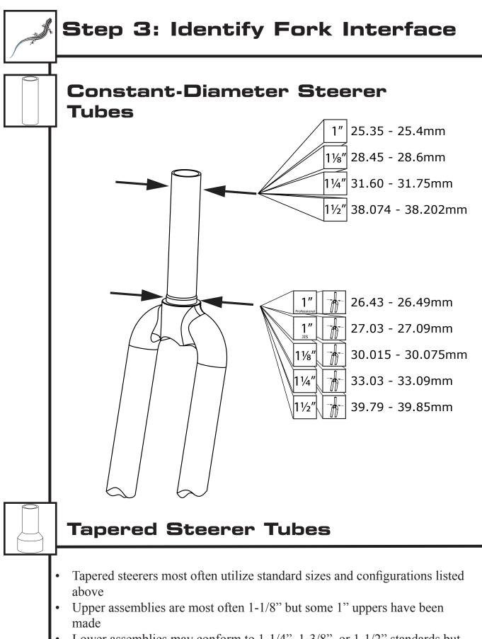
• Lower assemblies may conform to 1-1/4", 1-3/8", or 1-1/2" standards but many manufacturers use proprietary assemblies which makes identification and replacement more difficult.
