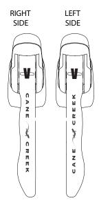
Fig. 1 - Install the brake lever onto the handlebar and depress the lever arm to access the internal mounting bolt.
